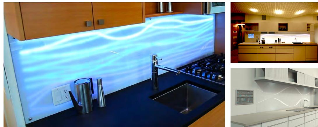
Ambient Canvas Prototypes [clockwise from left]: Version 2 in West House, Version 1 in North House, and a 3D rendering of the version 1 concept. Each prototype utilizes LED strings mounted behind a transmission medium (glass, acrylic, or Corian®) embedded in the kitchen backsplash.
